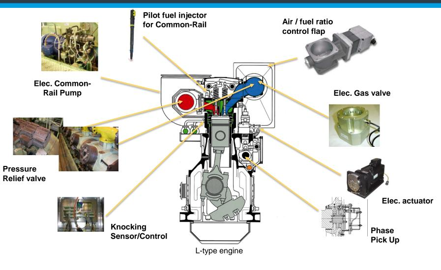
48/60 engines can be retrofitted to a 51/60DF engine
